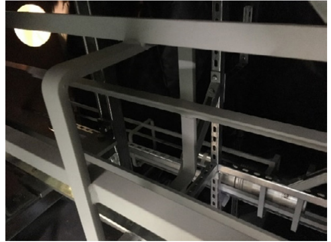
Figure 5: Image of an open rack storage system with SNM cannister visible in the bottom right hand corner.
